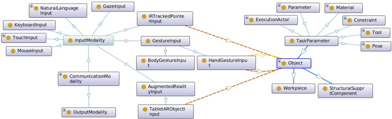
Fig. 3: Taxonomy of input modalities and task parameter types (blue arrows represent subclass relations). This excerpt shows that the input modalities *IRTrackedPointInput*, *HandGestureInput* and *TabletARObjectInput* provide values of parameter type *Object* (orange dashed arrows). The *preferredModality* (yellow dashed arrow) for this parameter type is set to be *HandGestureInput*.
