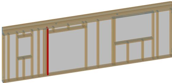
(b) Struts are manually assembled into wall structures.
