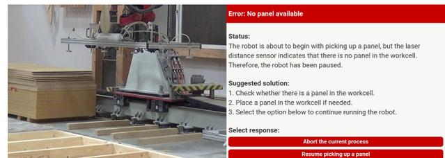
**Figure 10** Missing panel experiment: *left*: missing panel, *right*: semantic error message.
